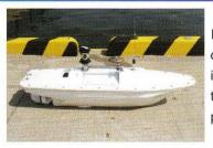
In no GPS reception area, collecting position information is possible by an auto tracking total station with 360 degree prism on board RC-S2.
