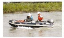
In the strong current and rushing river, towing RC-S2 by manned boat is good application. RC-S2 is all equipment in one survey boat.
